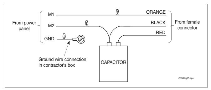
Figure 37. Wiring Schematic
