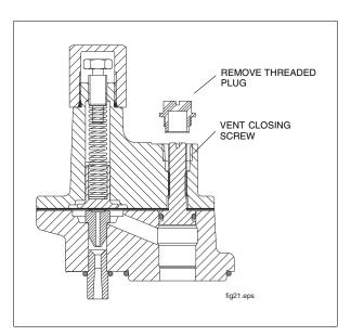
Figure 26. Closing The Check Valve
