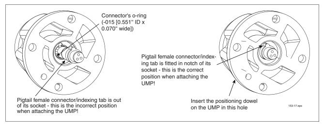
Figure 8. Verifying Pigtail's Female Connector Is Seated Properly
