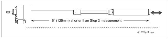
Figure 11. Adjusting Pump Length
