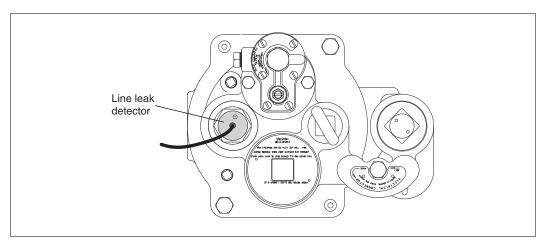
Figure 32. Electronic Line Leak Detector
