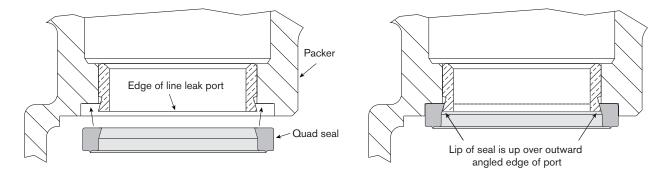
Figure 34. Installing New Quad Seal
