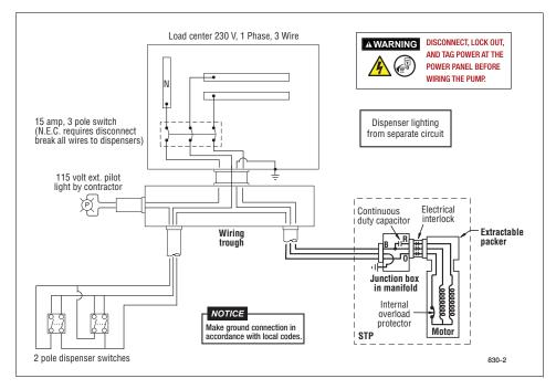
Figure 16. Suggested Wiring Diagram Without Optional Control Box
