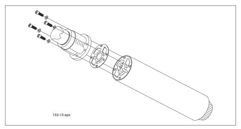
Figure 30. Replacing The gasket
