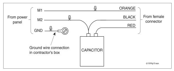
Figure 13. Capacitor Wiring Schematic
