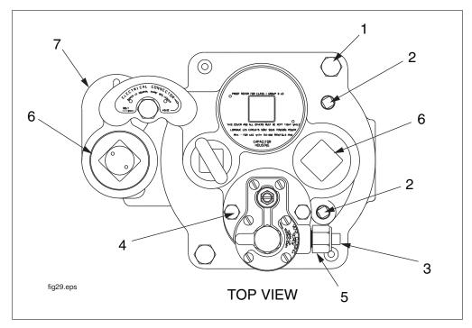
Figure 39. Packer-Manifold Assembly Top View - Part Identification
