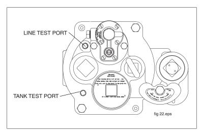
Figure 27. Line Test Port
