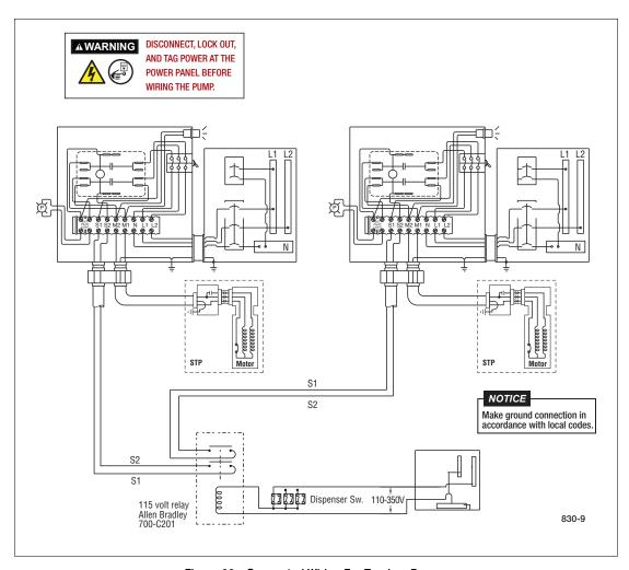
Figure 22. Suggested Wiring For Tandem Pumps
