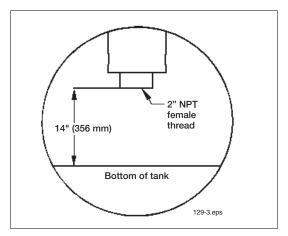
Figure 3. Floating Suction Adapter
