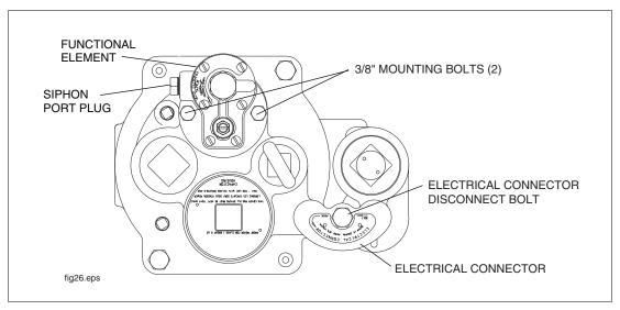
Figure 35. Packer With Functional Element
