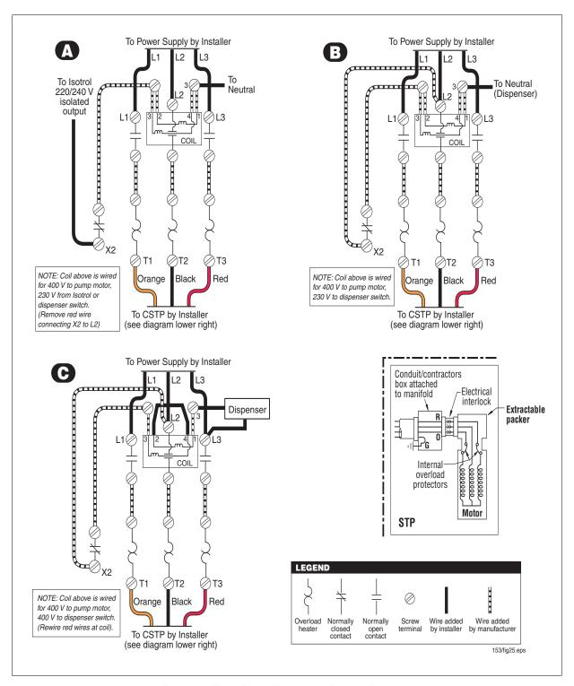
Figure 25. Three-Phase Pump Wiring Diagram Examples
