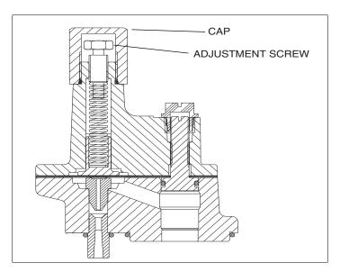
Figure 24. Functional Element Cap And Adjustment Screw
