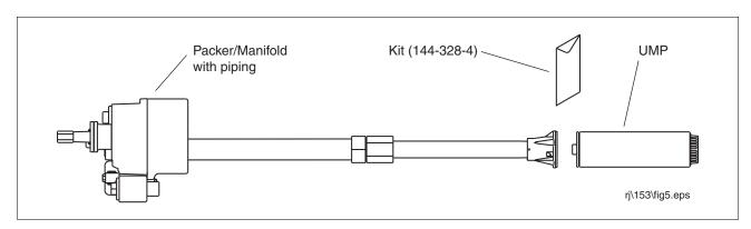
Figure 6. Packer/Manifold With Piping Attaching To UMP
