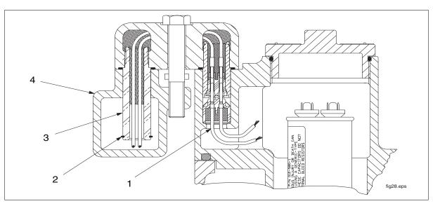
Figure 38. Yoke Assembly And Conduit Box Part Identification
