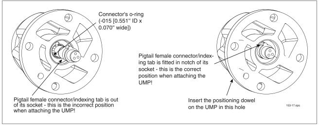
Figure 31. Verifying Pigtail's Female Connector Is Seated Properly
