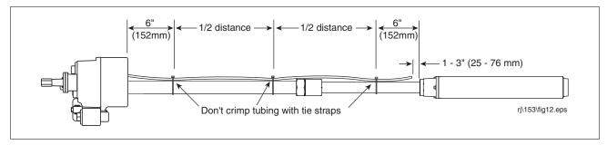
Figure 12. Attaching Return Line Tubing To Pump
