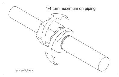
Figure 10. Loosening Locking Nut
