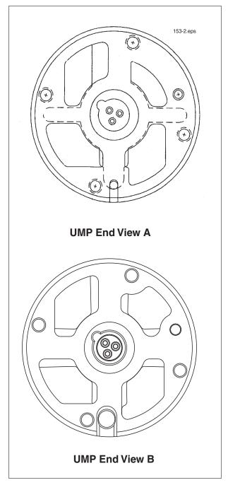
Figure 5. Identifying UMP Models By Their End View
