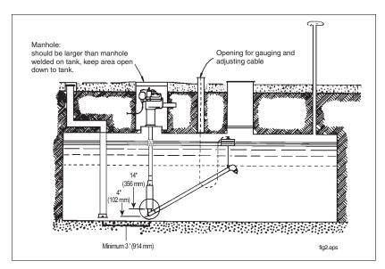
Figure 2. Floating Suction Installation
