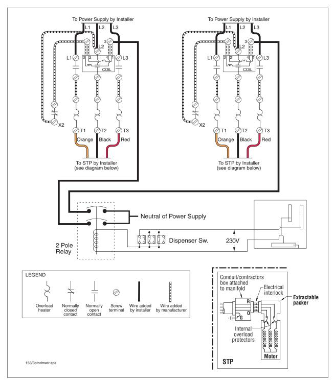
Figure 23. Suggested Wiring For Three-Phase Tandem Pumps
