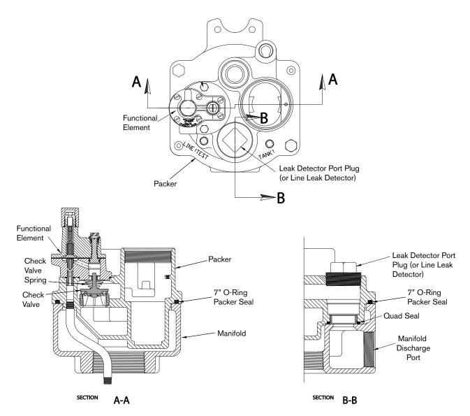
Figure 33. Locating 7" Packer O-Ring And Quad Seal
