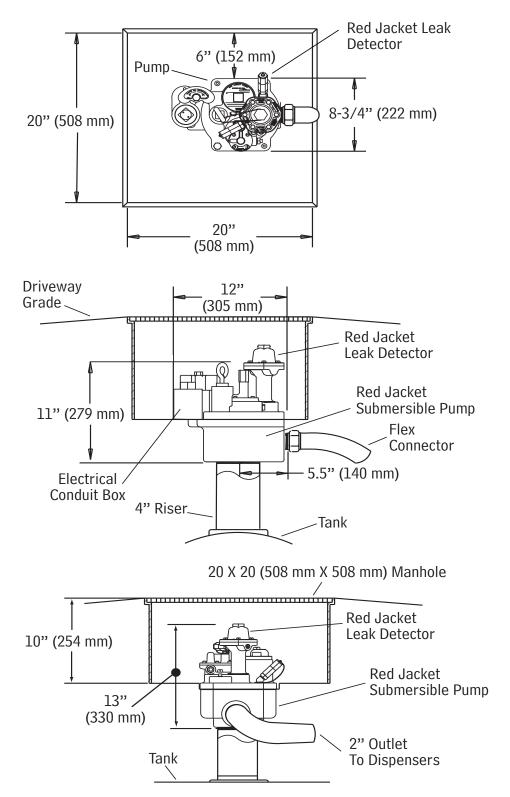
Figure 1. Leak Detector And Manifold Dimensions
