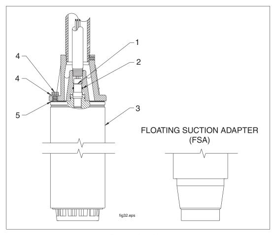
Figure 41. Pump Parts
