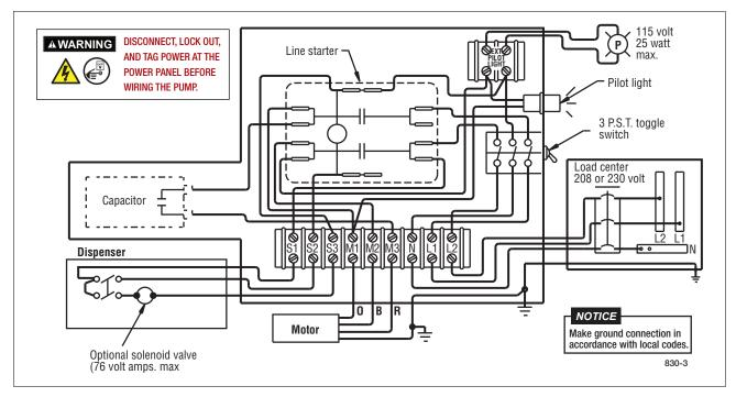
Figure 17. 230 Vac Remote Control Box With 110 VAC Coil And Cap - Model 880-045-5/880-046-5
