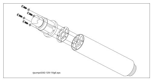
Figure 7. Aligning The UMP Gasket
